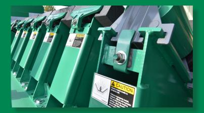
Richwood Impact Saddles® provide continuous support that protects the belt from tramp materials that can penetrate and rip the belt.
