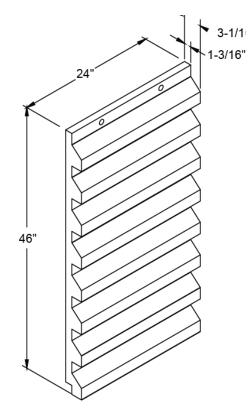
Wherever durable chute or bin linings are needed, count on Rock Flex<sup>®</sup> 2000 Profile Rubber Wear Plate. The profile step design presents the optimum angle of impact in vertical applications to achieve long wear life and effectively dissipate impact shock loads without damaging the body of the Wear Plate.
