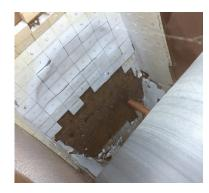
**Application**: Aggregates 3" minus granite. BEFORE: Ceramic liner proved too brittle and material destroyed the liner and the metal chute wall. Replacement required hanging in plates, boom trucks, torches and welders.
