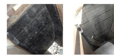
**Result**: Easier and safer installation, only worn pieces need replaced. Scheduling maintenance is simplified. Photo shown after three weeks run time.
